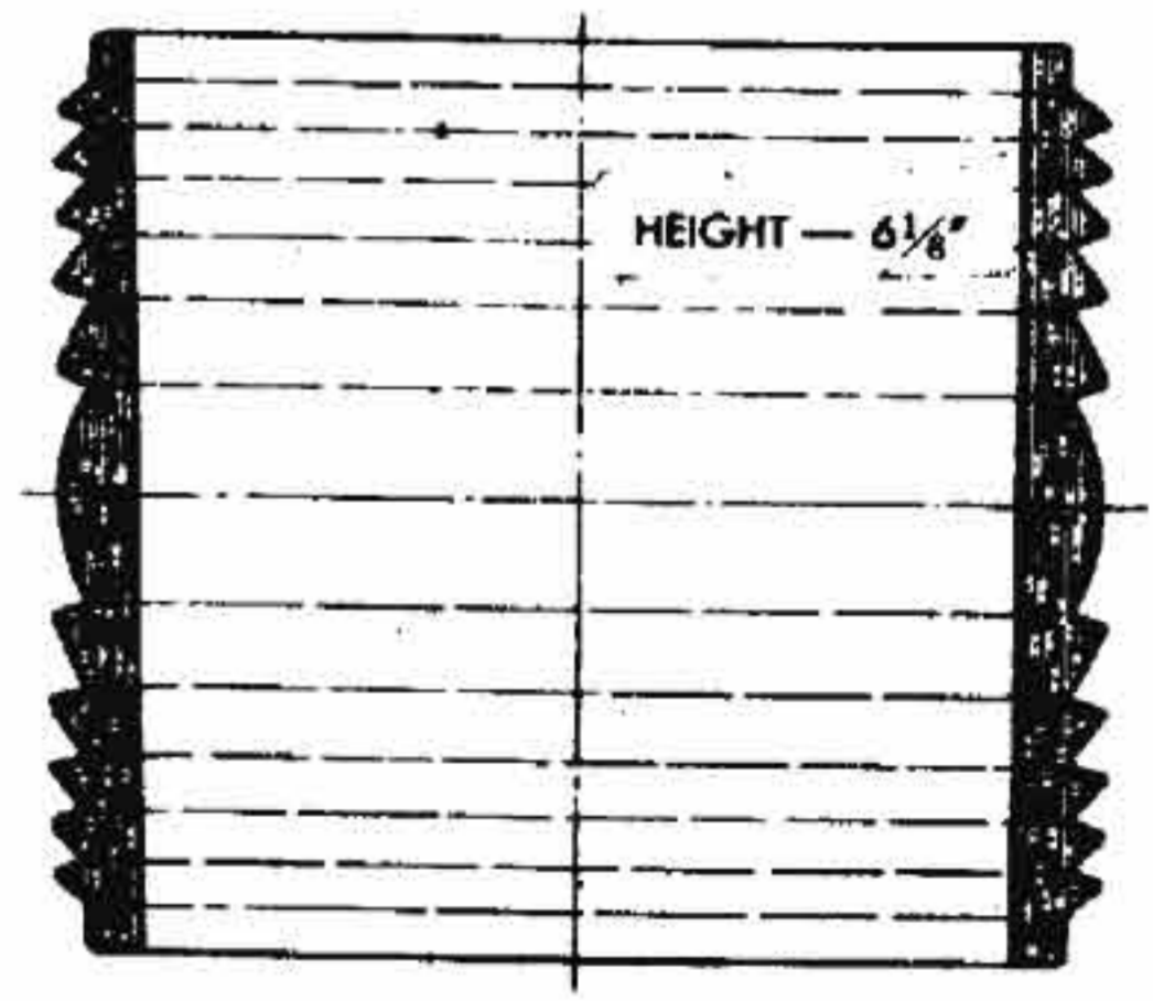
479-A1 150 mm PRESSED GLASS LENS
